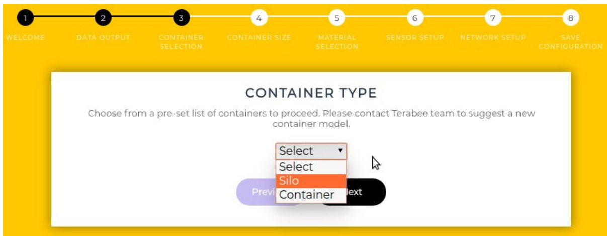
Figure 10 - Select the type of container you are going to use: Silo or Container (cuboid).
