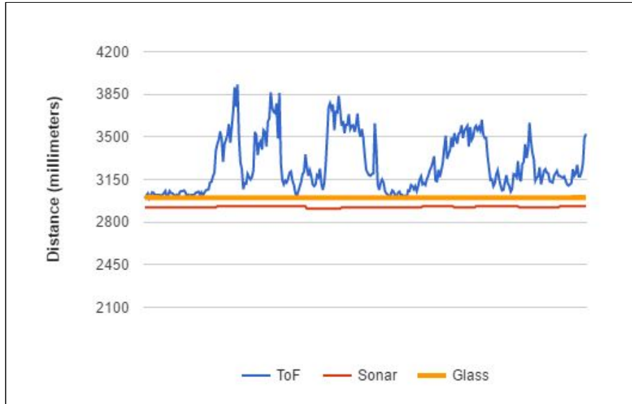
Figure 4.2 Surface: Metallic Coated Window
