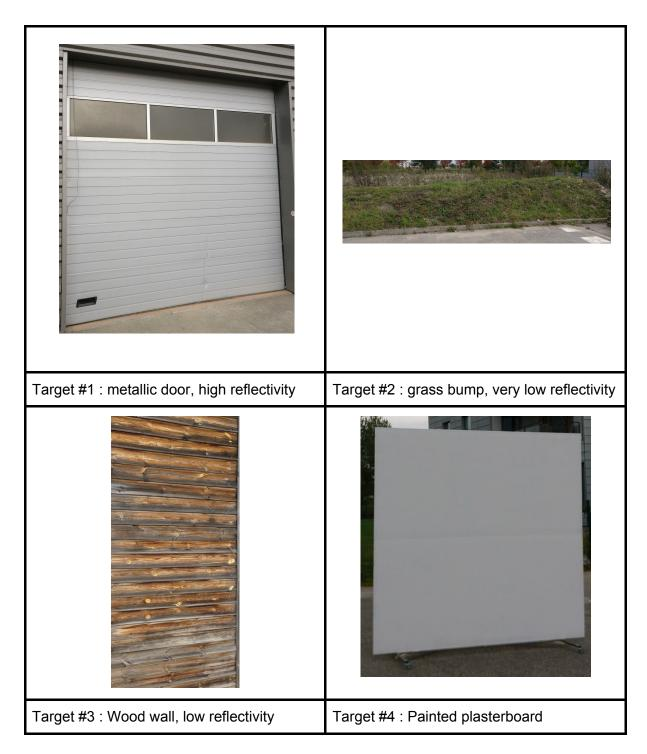
Note: Target #4 was built by Terabee as a control surface and was previously used in controlled indoor conditions. By taking it outdoors we were able to compare results with more random and potentially challenging lighting conditions.
