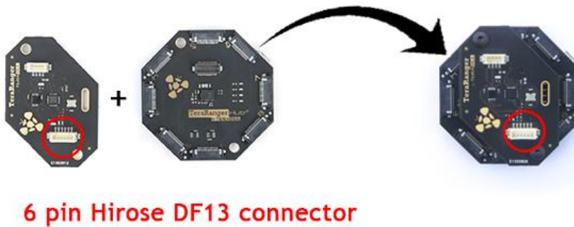
Figure 16. UART board connection to Hub Evo
