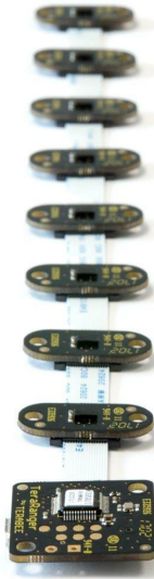
Figure 11. TeraRanger Multiflex PCB assembled
